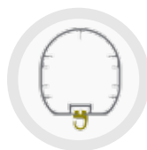
goal frame cross section 4,2" x 3,9"
